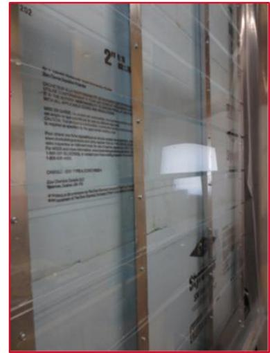
Figure 2: XPS test wall assembly
