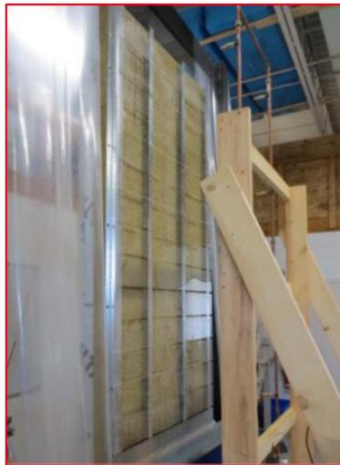
Figure 1: ROCKWOOL CAVITYROCK® DD test wall assembly
