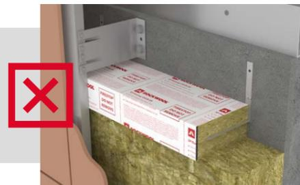
**TIP:** If suppliers of cladding systems are informed early in the design process for the rails, they are able to appropriately incorporate the locations of the horizontal barriers to ensure that the intumescent strip on the SP FireStop OSCB is free to expand to the rear of the cladding without obstruction.
