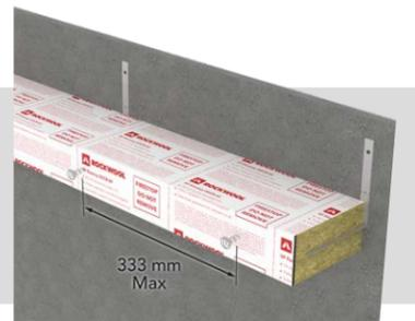
5. Ensure that the airspace does not exceed 25mm and that all of the pigtail screws are in contact with the cladding panel.
