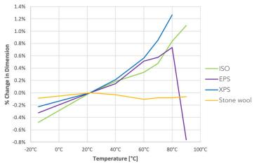
**Figure 10** Average Thickness Dimensional Changes for each Insulation Type
