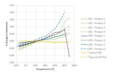
**Figure 8** Average Thickness Dimensional Changes for all Tested Products
