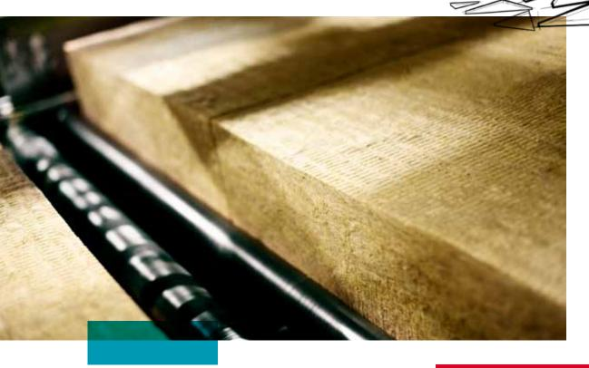
FABROCK™ Wrap is a light-density rolled stone wool insulation. It is engineered to be fabricated into OEM applications requiring insulation flexible enough to be wrapped around something while still maintaining its excellent fire, thermal and sound-absorbing properties.
