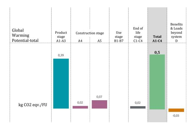
The main GWP contribution from the product life cycle is linked to the Product stage (A1-A3). This is primarily related to the materials delivered to the factory gate and consumption of electricity.
