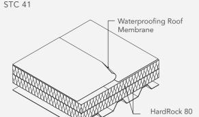
With the high density of ROCKWOOL HardRock roofing boards and the structure of the product, it provides the added mass necessary for effective sound insulation of membrane roof system. Additionally, the single-ply roof membrane coupled with ROCKWOOL stone wool insulation effectively minimizes rain impact noise on the roof system.
