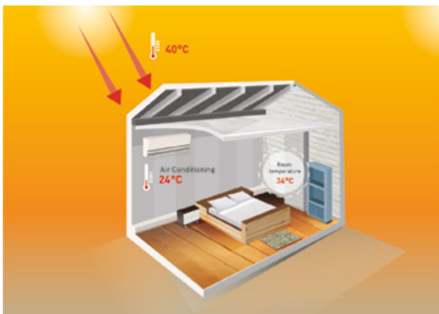
Diagram 2: Room without insulation requires 10°C cooling
