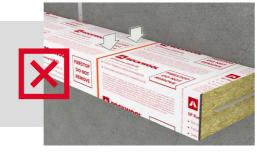
Ensure that the intumescent strip is free to expand to the rear of the cladding without obstruction, e.g. vertical cladding rails preventing free expansion.
