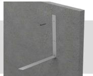
3. Impale OSCB onto the installed brackets at mid-depth, ensuring that the intumescent strip faces the open airspace. Ensure a tight butt joint between adjacent sections of barrier.
