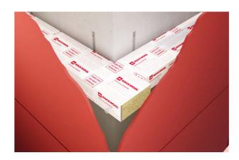
One run of OSCB oversails the other and is tightly butted against the cladding. The oversailing barrier should have a minimum bearing on the substrate of 200mm or 40% of the section length (whichever is greater), and should be supported by a minimum of two brackets.
