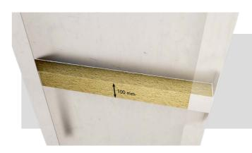
1. Cut a strip of ROCKWOOL SP FireStop Plus, 100mm in height, and compression-fit into the back of the cassette panel. The strip should be positioned appropriately so that it will be in line and centered with OSCB once the panel is installed.
