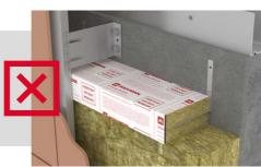
TIP: If suppliers of cladding systems are informed early in the design process for the rails, they are able to appropriately incorporate the locations of the horizontal barriers to ensure that the intumescent strip on the SP FireStop OSCB is free to to expand to the rear of the cladding without obstruction.
