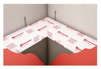
Internal: Internal corner joints should be mitred.
