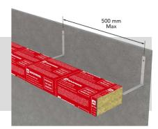
4. Ensure that the airspace does not exceed 44mm.
