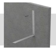
3. Impale OSCB onto the installed brackets at mid-depth, ensuring that the intumescent strip faces the open airspace. Ensure a tight butt joint between adjacent sections of barrier.
