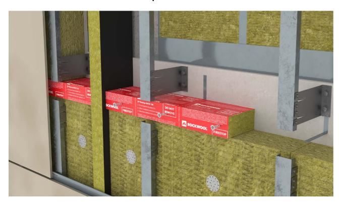
• Vertical runs of SP FireStop should be uninterrupted, with OSCB tightly abutting.
