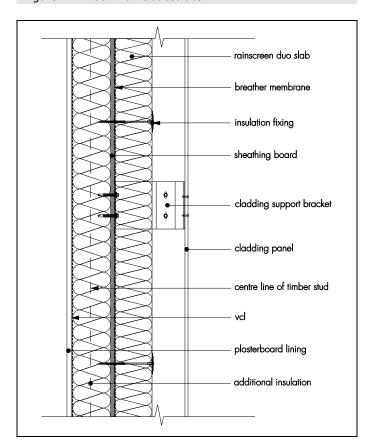
Figure 1 Timber Frame substrate
