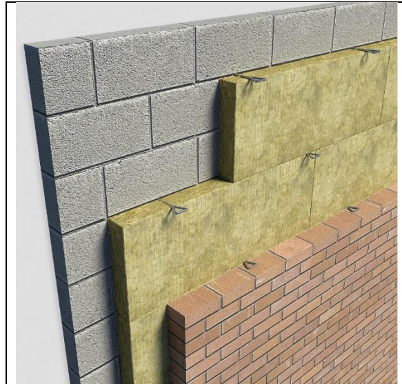
Figure 1 Wall tie positioning
