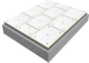
ROCKWOOL recommend the use of a plastic tube washer, or stress plate support thread when mechanically fastening roof boards to metal, concrete or timber deck warm roof systems. A stress plate and fastener fixings are required for ventilated timber deck cold roof systems.
