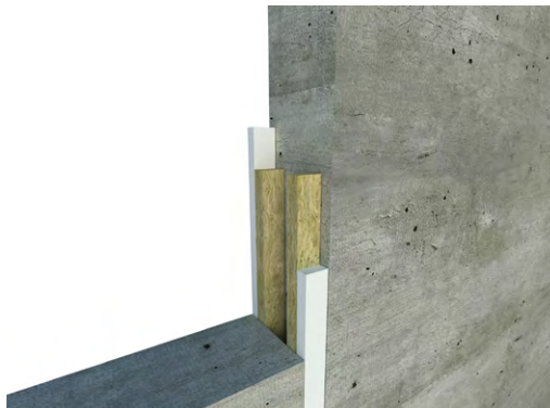
Figure 1 Double sealed joint with FirePro mineral wool backer
