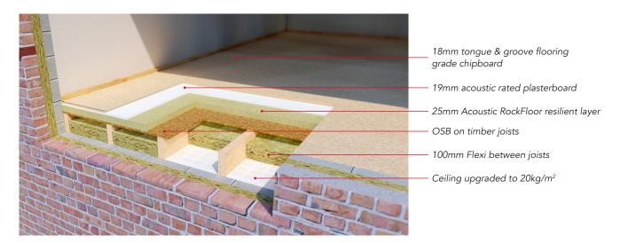
Note: If the existing ceiling is being replaced the sound performance of the floor can be further enhanced by fitting resilient bars which isolate the ceiling from the floor structure.
