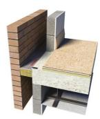
The external cavity should be stopped with ROCKWOOL SP 60 Firestop to minimise sound transmission along the cavity.
