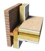
The external cavity should be stopped with ROCKWOOL TCB to minimise sound transmission along the cavity.
