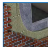
Masonry Cavity Walls Thermal Cavity Batt
