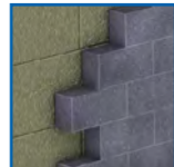
Masonry Party Walls Thermal Cavity Batt
