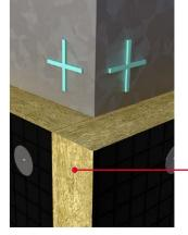
Board edges must be covered with ROCKWOOL Black Foil Tape
