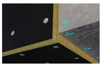
Figure 3 Cross joint horizontal duct
