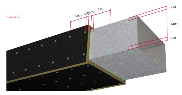
Side wall slabs must overlap the top and bottom boards as shown in Figures 3 & 4. All cross joints must be bonded with ROCKWOOL FIREPRO® Glue.
