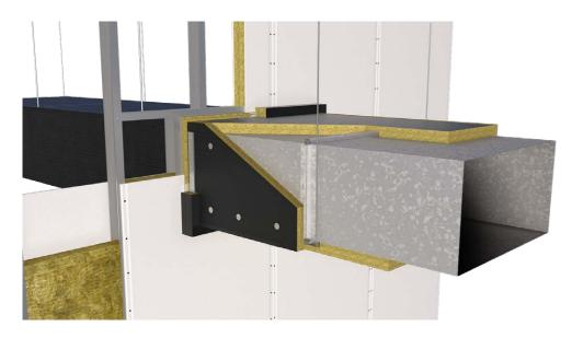
Figure 8 ROCKWOOL Patented Dry Wall Penetration Detail
