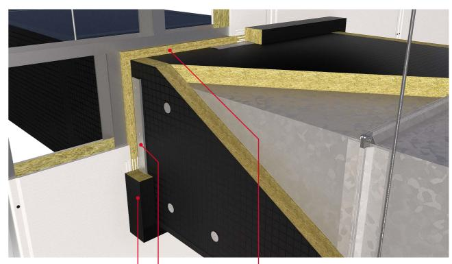
60mm x 100mm DuctRock collars bonded to the substrate with FIREPRO<sup>®</sup> Glue
