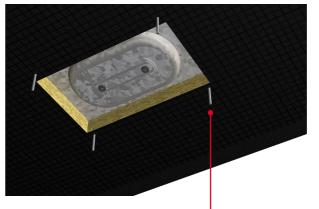
4 x M8 threaded rods secured to both sides of the duct.
