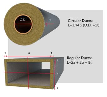
Indicative thickness of insulation for ductwork carrying warm air to control heat loss (taken from BS5422:2009 Table 13) Horizontal duct @ 35°C, still air @ 15°C
