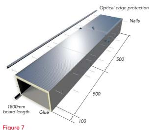
Rectangular ducts – 45° mitre joint system, showing installation sequence
