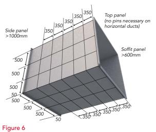
Steel pin arrangement where side panel is greater than 1000mm or soffit panel is greater than 600mm
