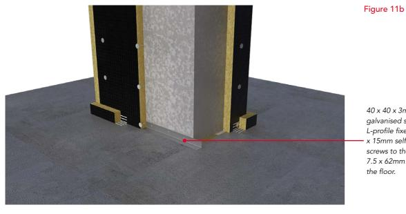
40 x 40 x 3mm galvanised steel L-profile fixed with 3.2 x 15mm self tapping screws to the duct and 7.5 x 62mm screws to the floor.
