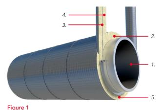
Fire Duct Section applied to circular duct
